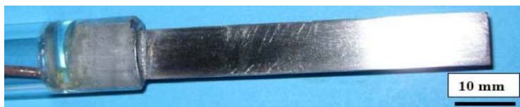
Figure 4: X65 test electrode
